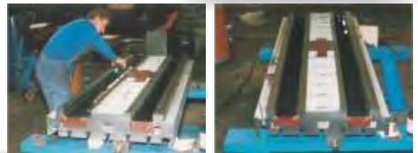
moulding of flat ways by pouring
