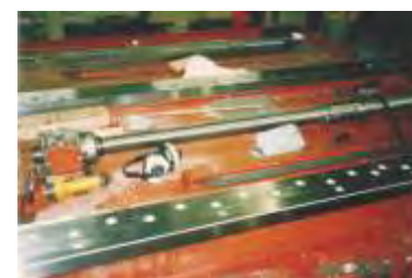
adjustment of linear slideways
